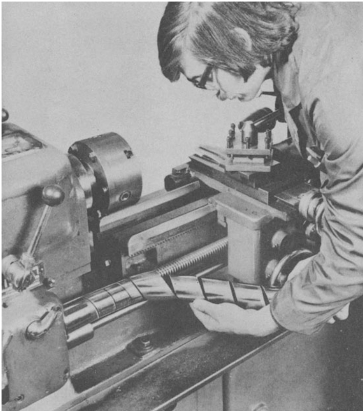
Photo 2 A 'Tensaguard' safety cover being fitted to a lathe (Photograph courtesy of Tensator Limited)
