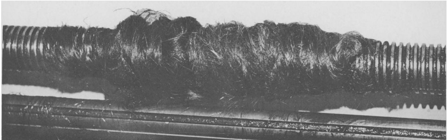
Photo 1 The horrifying effects of catching long hair in a lathe leadscrew
