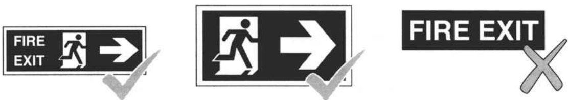
Fig. 1.6 Text only safety signs do not comply.
