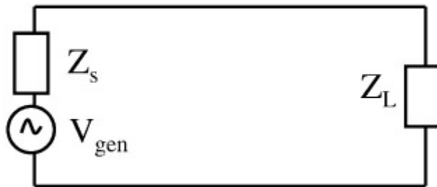
Figure 10.2: Nonideal loop that contains impedances.
