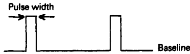
Figure 1.13 The width of a pulse is the time for which the important part of the pulse is at a steady voltage.
