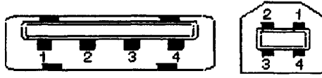
Figure 9.5 The two main types of USB sockets used on current models of computers and peripherals.
