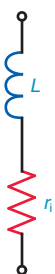
Figure 19–33 The internal dc resistance r_i of a coil is in series with its inductance L .
