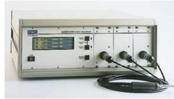
Figure 13–15 A gaussmeter to measure flux density, with a probe containing an indium arsenide element.
