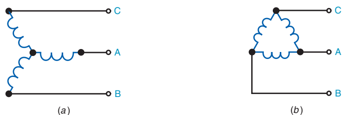
Figure 15–26 Types of connections for three-phase power. (a) Wye or Y. (b) Delta or \Delta .
