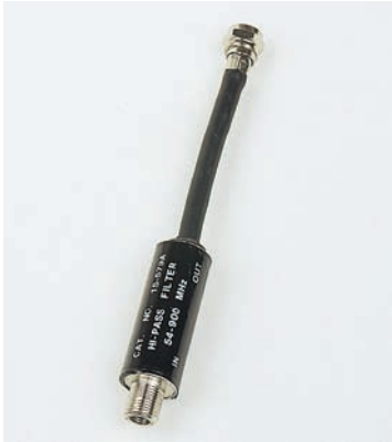
Figure 26–29 A television antenna filter to pass TV channel frequencies above 54 MHz but attenuate lower frequencies that can cause interference
