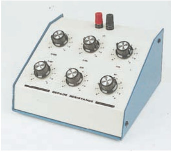
Figure 2-16 Decade resistance box for a wide range of R values.
