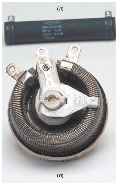
Figure 2-3 Large wire-wound resistors with 50-W power rating. (a) Fixed R , length of 5 in. (b) Variable R , diameter of 3 in.
