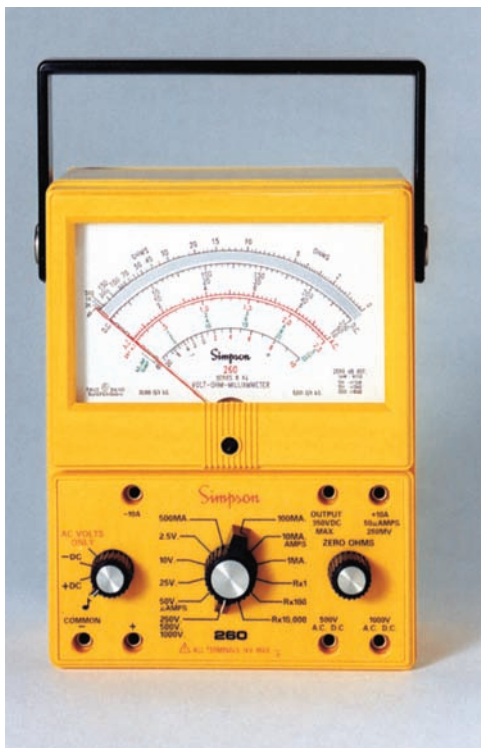
Figure 8–13 Analog VOM that combines a function selector and range switch.
