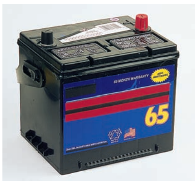
Figure 12–2 Example of a 12-V auto battery using six lead-acid cells in series. This is a secondary type, which can be recharged.
