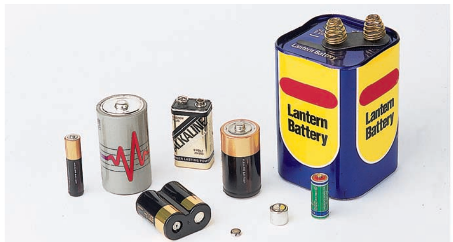
Figure 12–1 Typical dry cells and batteries. These primary types cannot be recharged.
