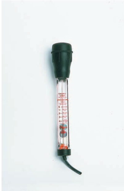
Figure 12–9 Hydrometer to check specific gravity of lead-acid battery.
