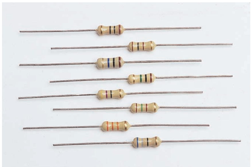
Figure 2–2 Carbon resistors with same physical size but different resistance values. The physical size indicates a power rating of 1/2\ W .
