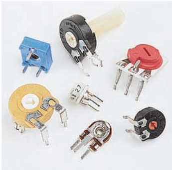
Figure 2-19 Small potentiometers and trimmers often used for variable controls in electronic circuits. Terminal leads are formed for insertion into a PC board.
