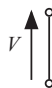
Figure 3.8 A short-circuit. The voltage V between the terminals is zero whatever the value of the current through it
