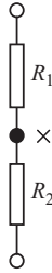
Figure 3.18 The series connection of two resistors. Note that there is nothing else connected to point X
