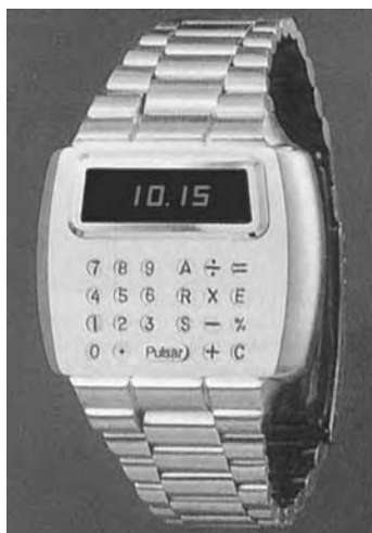
Fig. 1.8. Pulsar calculator watch with LED display released in 1975 by Hamilton Corporation. The first Pulsar LED watch (without calculator) was offered in 1972. It was based on GaInP LEDs (after Seiko, 2004).
