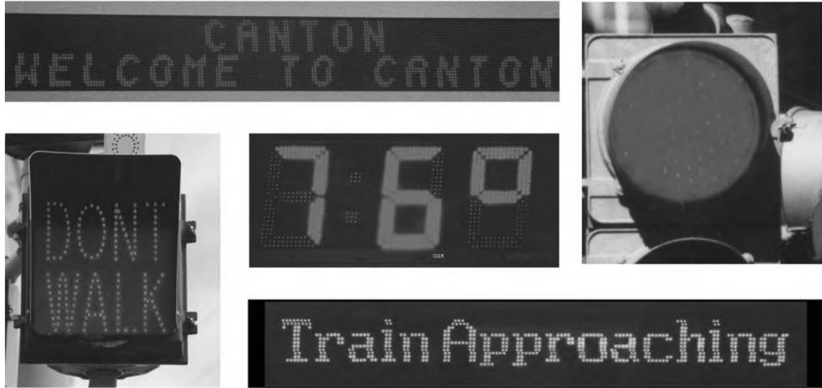
Fig. 1.13. Examples of red and amber AlGaInP/GaAs LEDs used in signage applications.
