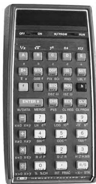
Fig. 1.9. Programmable pocket calculators Model SR-56 of the Texas Instruments Corporation and Model HP-67 of the Hewlett-Packard Corporation, both first manufactured in 1976. Seven-segment numeric characters composed of GaAsP LEDs were used in the display. The SR-56 came with a “huge” program memory of 100 steps. The HP-67 came with a magnetic card reader and had several freely programmable keys.
