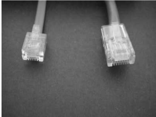
RJ 45 connector (right). RJ 11 (left)
