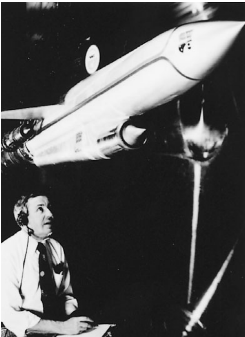
Figure 5.6 Some of the most beneficial research with physical models has been accomplished with wind tunnels. Here a ram jet model is being studied in a 10 ft. \times 10 ft. test section. (Courtesy of the National Aeronautics and Space Administration.)
