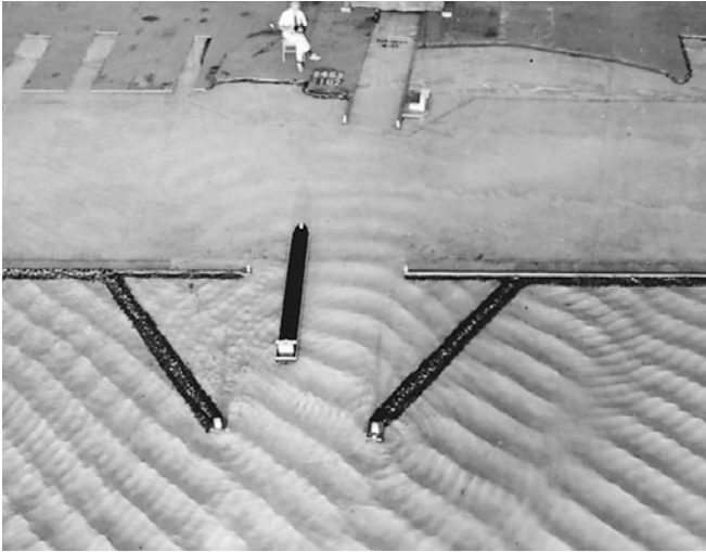
Figure 5.5 A physical model used to study the behavior of waves in a harbor. (Courtesy of the U.S. Army Corps of Engineers.)
