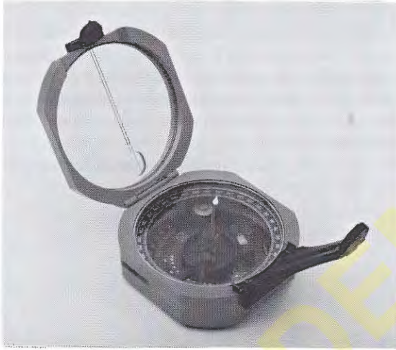
Figure 2.11 A Brunton compass is used to measure bedrock attitudes and other geologic features in the field.
