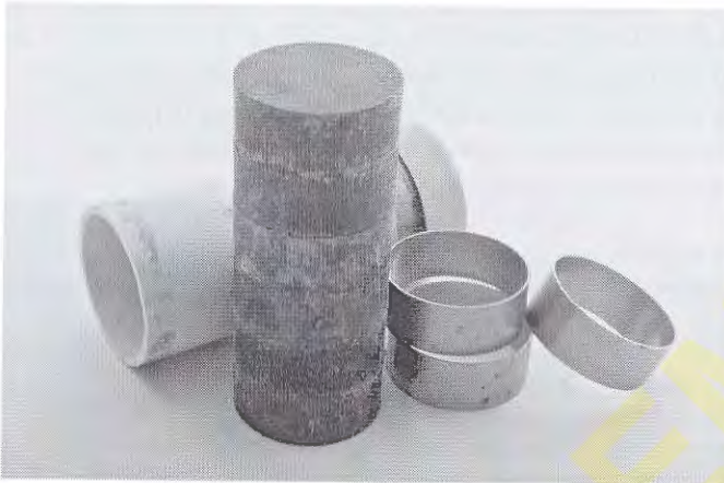
Figure 3.20 Soil samples from heavy-wall samplers are contained in liners and stored in plastic tubes. In this case, the liners have an outside diameter of 2.5 in, a height of 1.0 in, and are made of brass.
