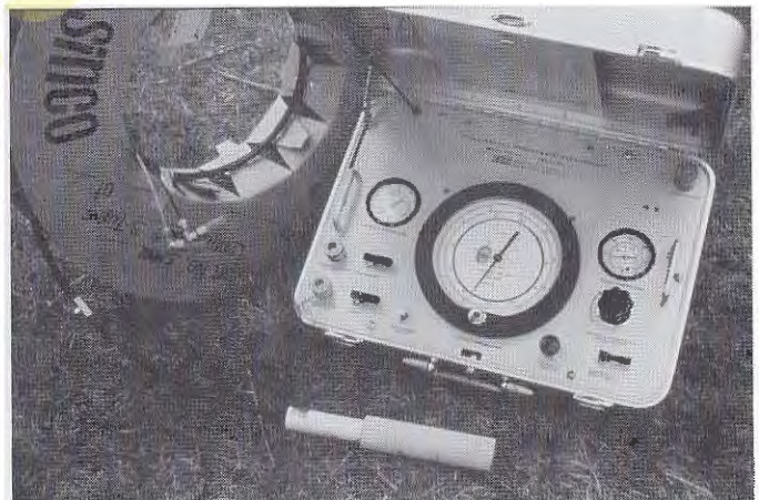
Figure 7.8 A pneumatic piezometer and readout unit. (Slope Indicator Co.)
