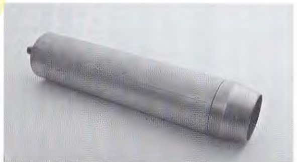
Figure 3.19 A heavy-wall sampler. (a) Cross-section showing liners. The dimensions shown are typical, but many different sizes are used. (b) The sampler can be opened to retrieve the liners, and thus is often called a split barrel sampler . The liners are available in different lengths.
