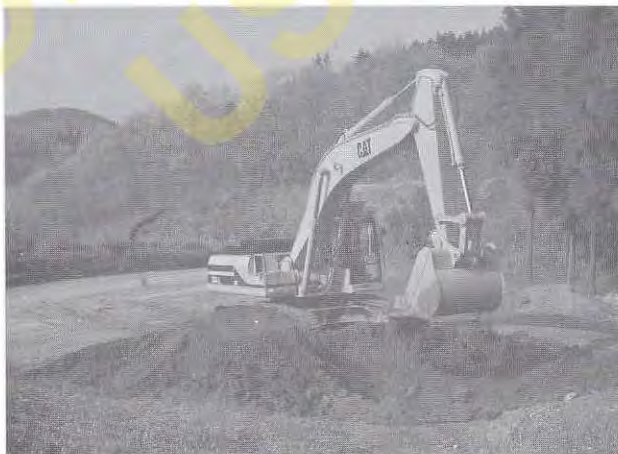
Figure 6.9 An excavator is a large hoe mounted on a special rotating chassis. This excavator is digging a hole on the right side of the picture and dumping the spoils in a pile on the left side. Excavators also can dump directly into trucks. (Caterpillar Inc.)
