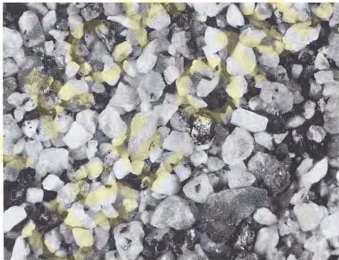
Figure 4.1 Microphotograph of a medium sand at 5 \times magnification.
