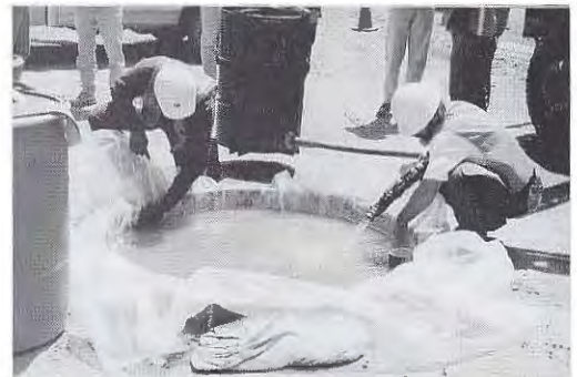
Figure 6.36 Use of a water ring test to assess compaction in an earth dam with cobbles and boulders: a) Hole has been dug and excavated soils have been weighed; b) Hole has been lined with plastic and filled with water to measure its volume.
