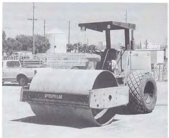
Figure 6.22 Self-propelled vibratory roller.
