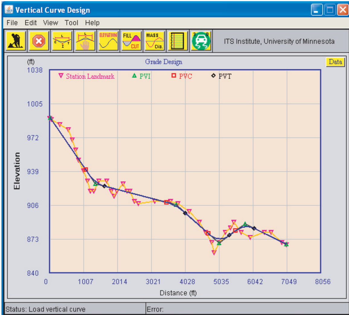
FIGURE 5 Roadway geometry design—vertical design.
